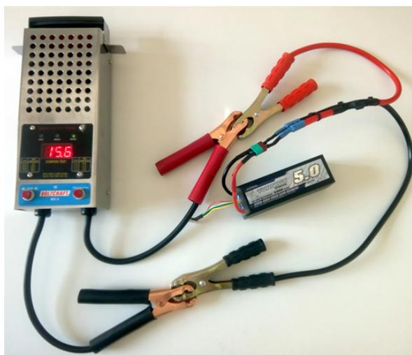
Fig 1. Depiction of the cold jump start test
