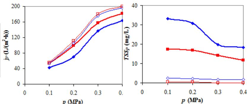
Fig. 3. Permeate flux and permeate TSS vs. operating pressure for different feed flow rates of untreated ( $TSS_F=60$  mg/L) and pretreated ( $TSS_F=15$  mg/L) ARW (untreated:  $\blacklozenge G_V=7$  m<sup>3</sup>/h,  $\blacksquare G_V=10$  m<sup>3</sup>/h; pretreated:  $\diamond G_V=7$  m<sup>3</sup>/h,  $\square G_V=10$  m<sup>3</sup>/h)
