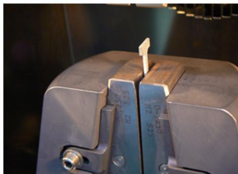
Fig.2. The test specimen in the Instron testing machine
