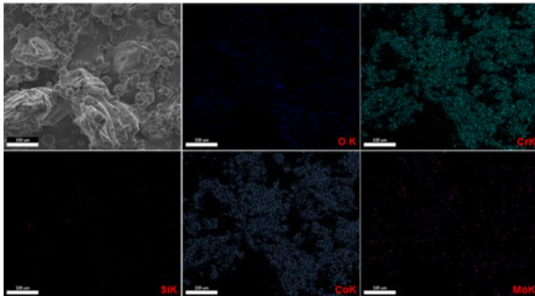
Fig. 3. EDAX mapping distribution of principals chemical elements over the laser-sintered material scanned area
