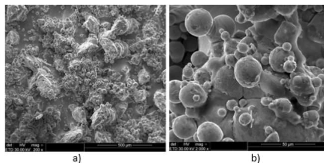
Fig. 1. SEM micrographs of melted EOS CobaltChrome MP1 alloy powder: a - magnification by 200x; b - magnification by 2000x
