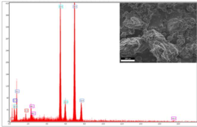
Fig. 2. The energy dispersive x-ray spectra of the laser-sintered Co-Cr powder surface test sample
