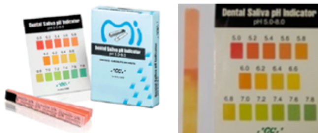
Fig. 3. GC Saliva pH Indicator used in study (left); salivary chart indicating a pH value of 6.2 for the used strip (right)
