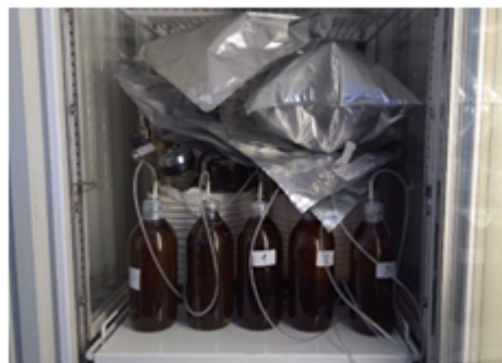
Fig. 1. Laboratory experimental set-up for the anaerobic digestion tests
