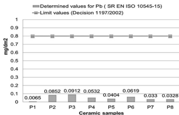
Fig. 6. Lead given off by glazed tiles
