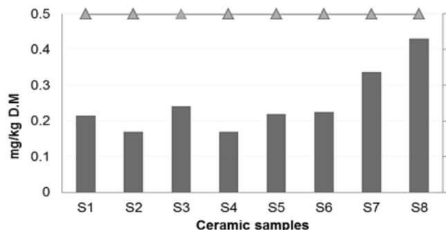
Fig. 2. Leaching tests for ceramic samples - total chromium
