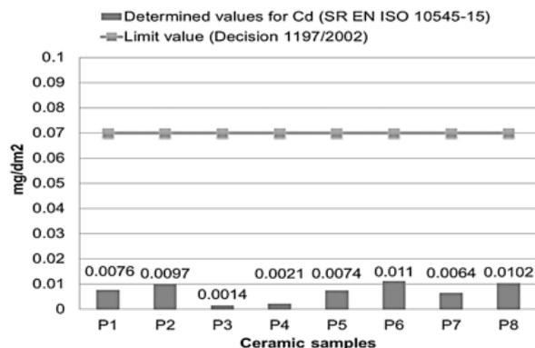
Fig. 5. Cadmium given off by glazed tiles
