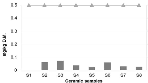
Fig. 3. Leaching tests for ceramic samples - lead
