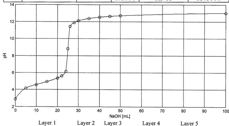
Fig. 1. Titration curve for weak acid with strong base
