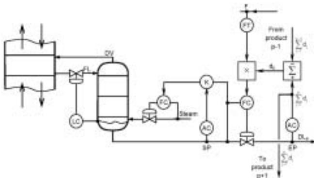
Fig. 4. Alternative control structure for  $p$  sideproduct [1]
