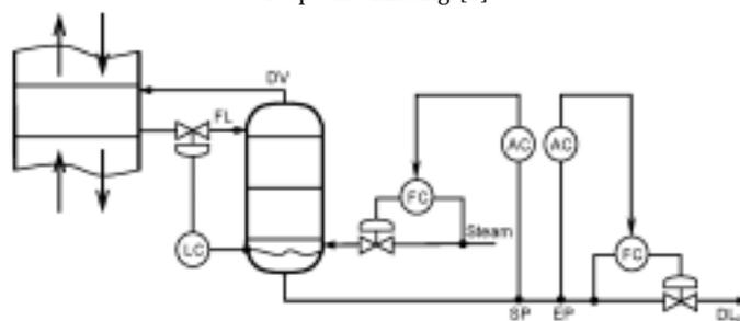
Fig. 2. Control structure for  $p$  sideproduct, with simple quality control loops [1]
