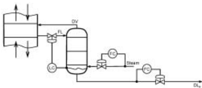
Fig. 1. Classical control structure for  $p$  sideproduct. Quality control loops are missing [1]
