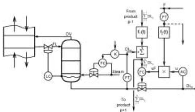
Fig. 3. Shinsky control structure for  $p$  sideproduct [1]
