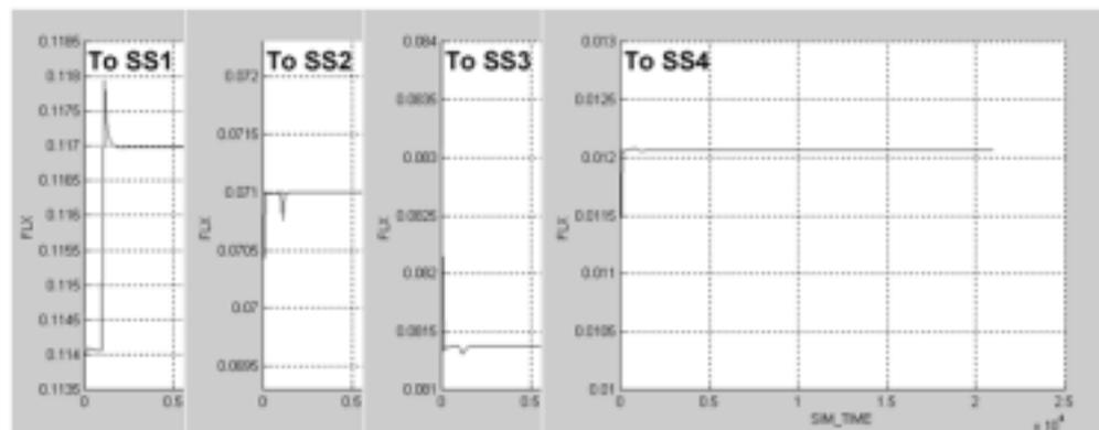
Fig. 7. Plant response for a 0.23 to 0.26 increase in reflux ratio, with the dynamic decoupler connected. Liquid sidedraws to SS1, SS2, SS3 and SS4 flowrates are presented in [kmol/s]. The simulation time is expressed in  $[s \times 10^4]$ .
