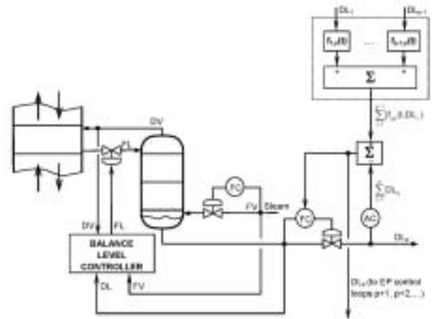
Fig. 5. Original control structure for  $p$  sideproduct, with quality loops dynamic decoupling [1]
