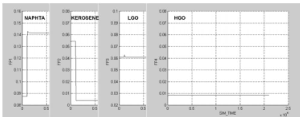
Fig. 10. Plant response for a 0.09 kmol/s to 0.14 kmol/s increase in naphtha flowrate, with the dynamic decoupler connected. Naphtha, kerosene, LGO and HGO flowrates are presented in [kmol/s]. The simulation time is expressed in [s × 10<sup>4</sup>].
