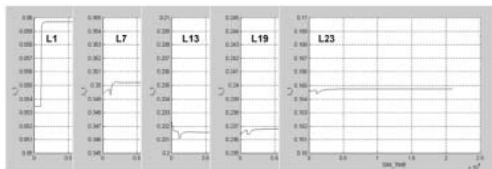
Fig. 8. Plant response for a 0.23 to 0.26 increase in reflux ratio, with the dynamic decoupler connected. Internal reflux from trays 1, 7, 13, 19 and 23, in [kmol/s], are depicted. The simulation time is expressed in  $[s \times 10^4]$ .
