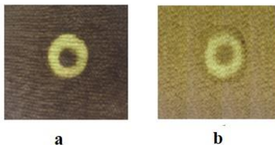
Figure 1. Photochemical films on tissue samples from the side facing the solar radiation (a) and from the opposite side (b)
