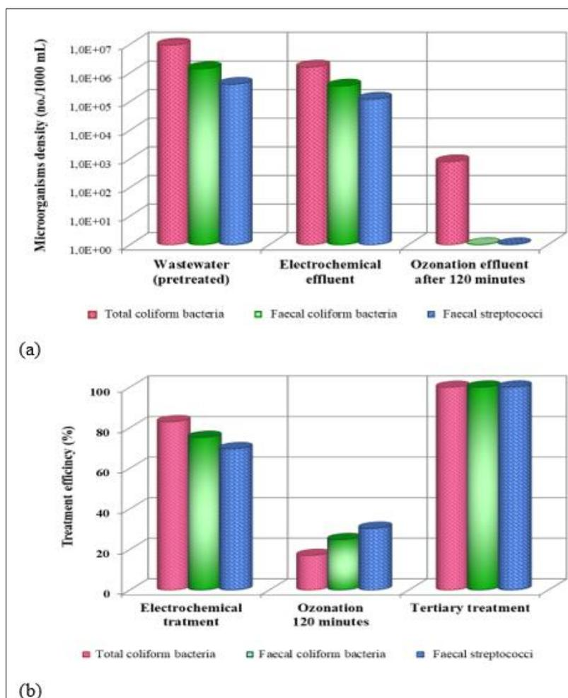
**Figure 3.** Removal of microorganisms from wastewater
