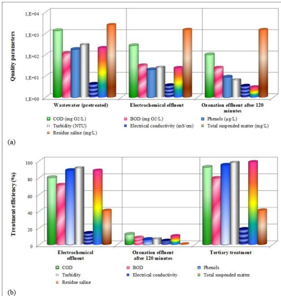
**Figure 2.** Removal of organic substances, suspended matter and salts from wastewater
