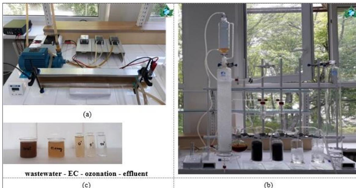
**Figure 1.** Experimental set-up for the advanced (tertiary) wastewater treatment: (a) electrocoagulation step ; (b) ozonation step ; (c) the variation of colour of treated wastewater
