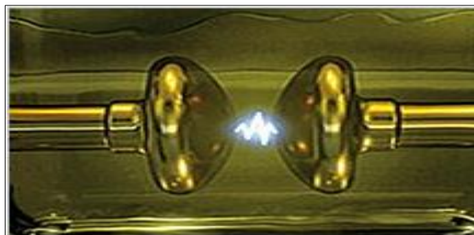
Figure 4. Voltage breakdown during sample oil testing
