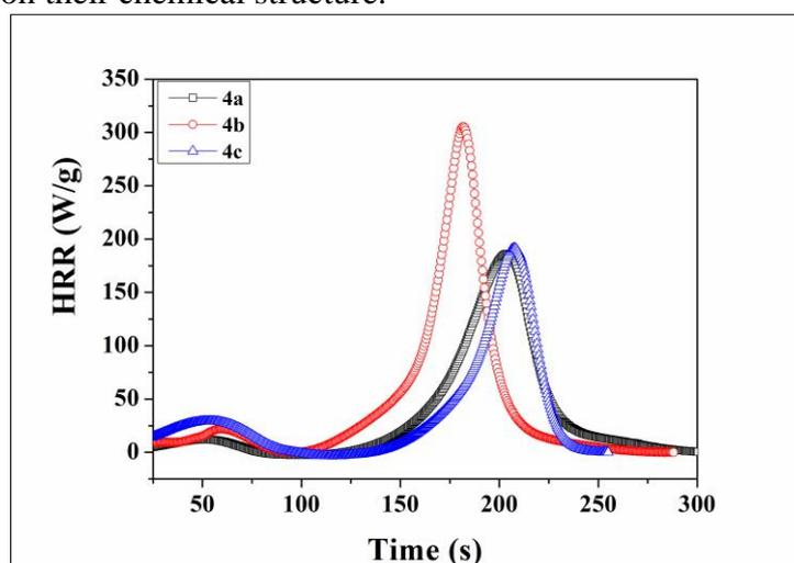
**Figure 4.** The HRR curves for the phosphorus-containing polyimide **4**
