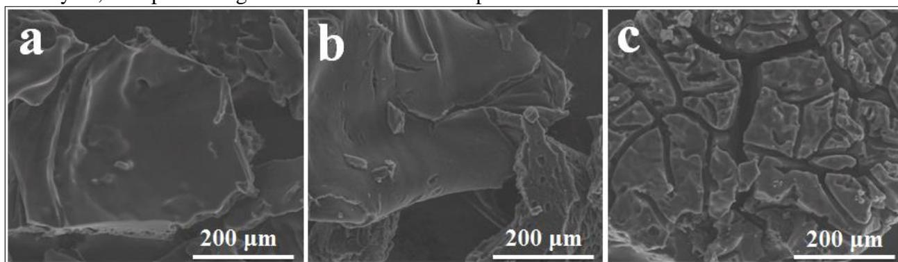
**Figure 5 .** SEM images of the char yield for the phosphorus-containing polyimides **4**
