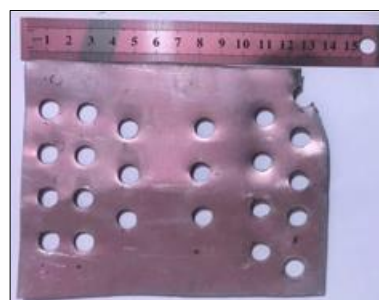
Figure 3. Aluminum electrode after electrocoagulation
