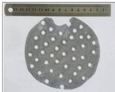
Figure 2. Iron electrode after electrocoagulation
