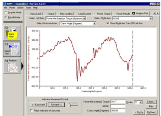
Fig. 3. The variation of the motor moment at the crankshaft during the stroke 71
