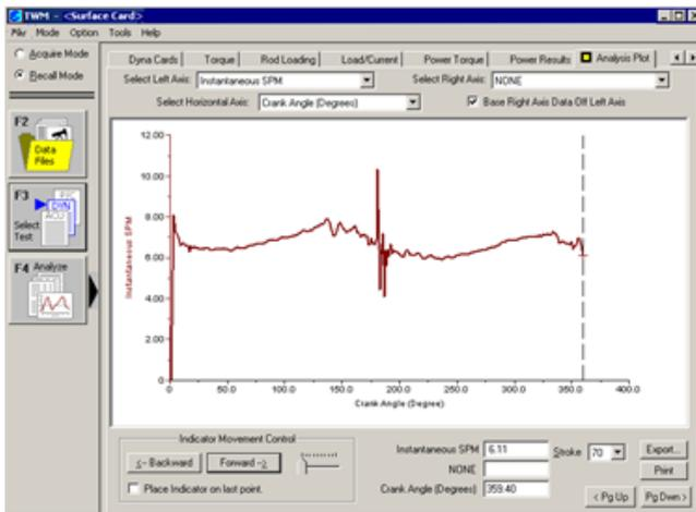
Fig. 2. The variation of the angular speed of the cranks expressed in rot/min during the stroke 70
