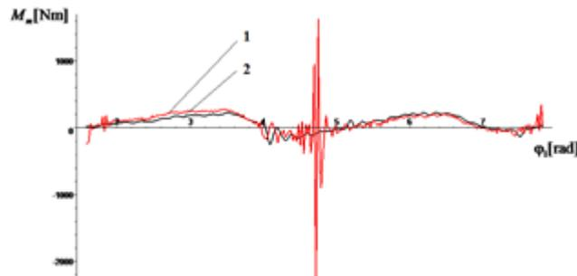
Fig. 9. The variation of the motor moment at the crankshaft during the stroke 71 (simulation - curve 1; experimental - curve 2)
