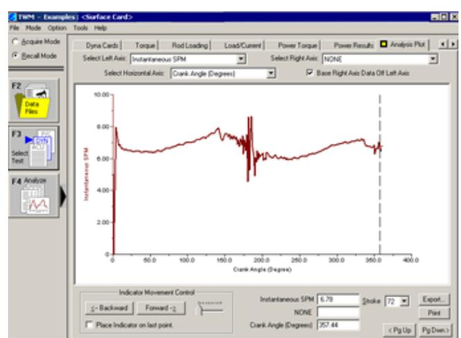
Fig. 6. The variation of the angular speed of the cranks during the stroke 72
