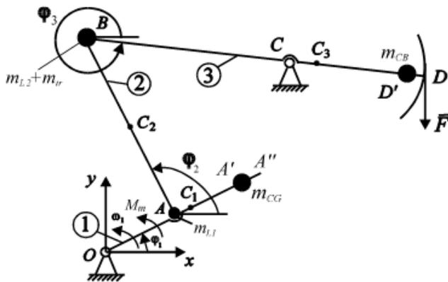
Fig. 7. The mechanism of the conventional pumping units
