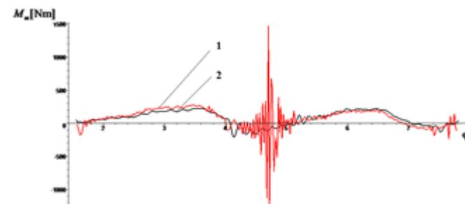
Fig. 10. The variation of the motor moment at the crankshaft during the stroke 72 (simulation - curve 1; experimental - curve 2)
