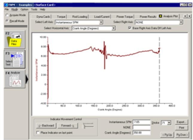
Fig. 5. The variation of the angular speed of the cranks during the stroke 71
