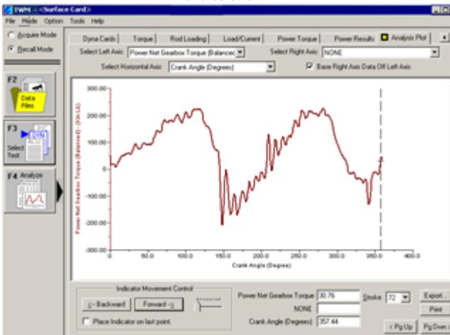
Fig. 4. The variation of the motor moment at the crankshaft during the stroke 72
