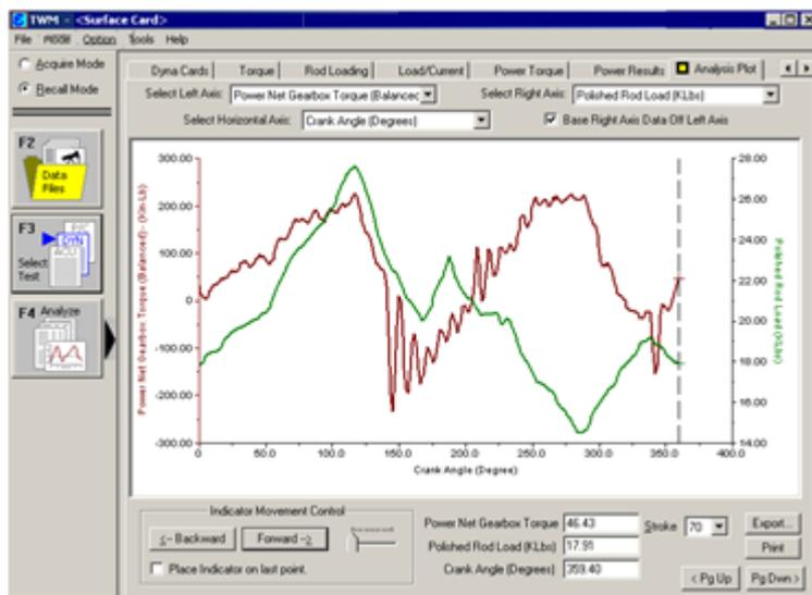
Fig. 1. The variation of the force at the polished rod and of the motor moment at the crankshaft during the stroke 70
