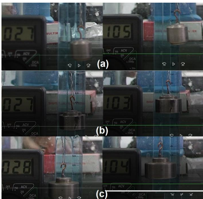
Fig. 6. Load-lifting by work-generating SME performed by a ring shaped specimen (0.7 g) cut from a multi-layered PET heat-shrinkable sheath: (a) for a 270 g load; (b) for a 590 g load and (c) for a 1100 g load
