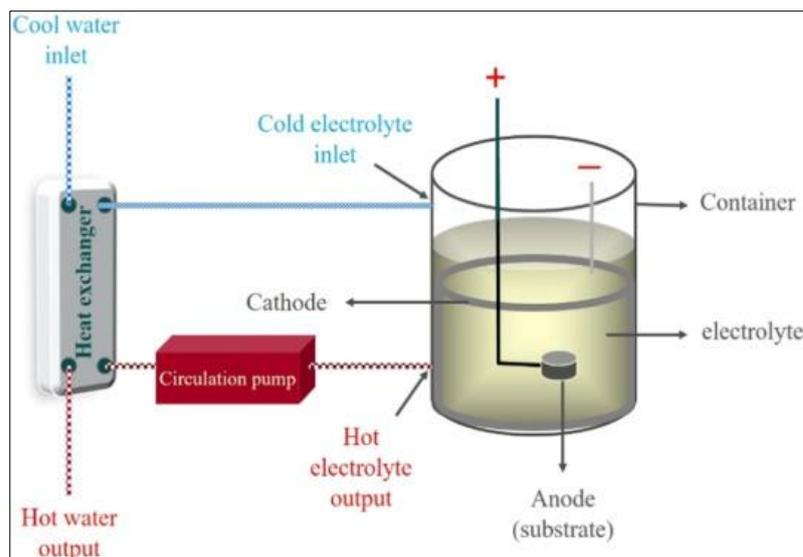
**Figure 4.** Ceramic coatings using micro arc oxidation method [23]
