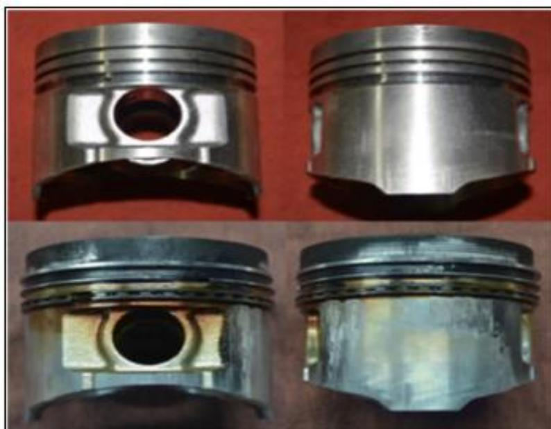
Figure 2. Ceramic coated piston [13]
