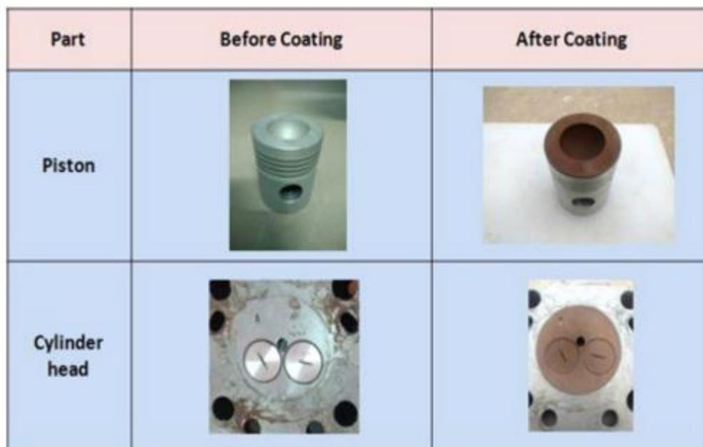
**Figure 3.** Piston, and Combustion chamber coated by plasma coating technique [24]
