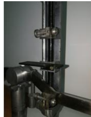
b) Wire clamping mode in testing of wire rods
