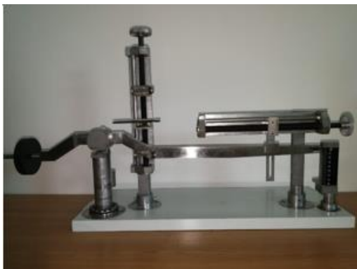
a) Experimental device for wire tensile testing
