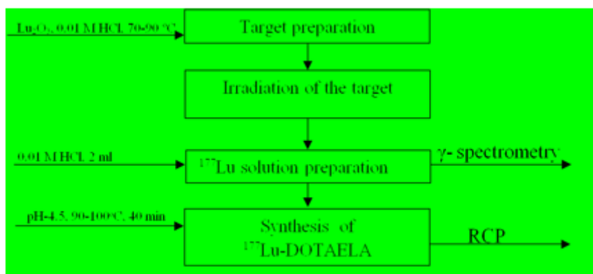
Figure 3. The technological scheme for ^{177}\text{Lu} -DOTAELA production
