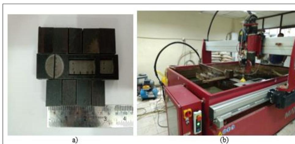
**Figure 1.** a) Pockets in AISI 1045 with Square, Rectangle, and Circle, b) Abrasive water jet machining set up
