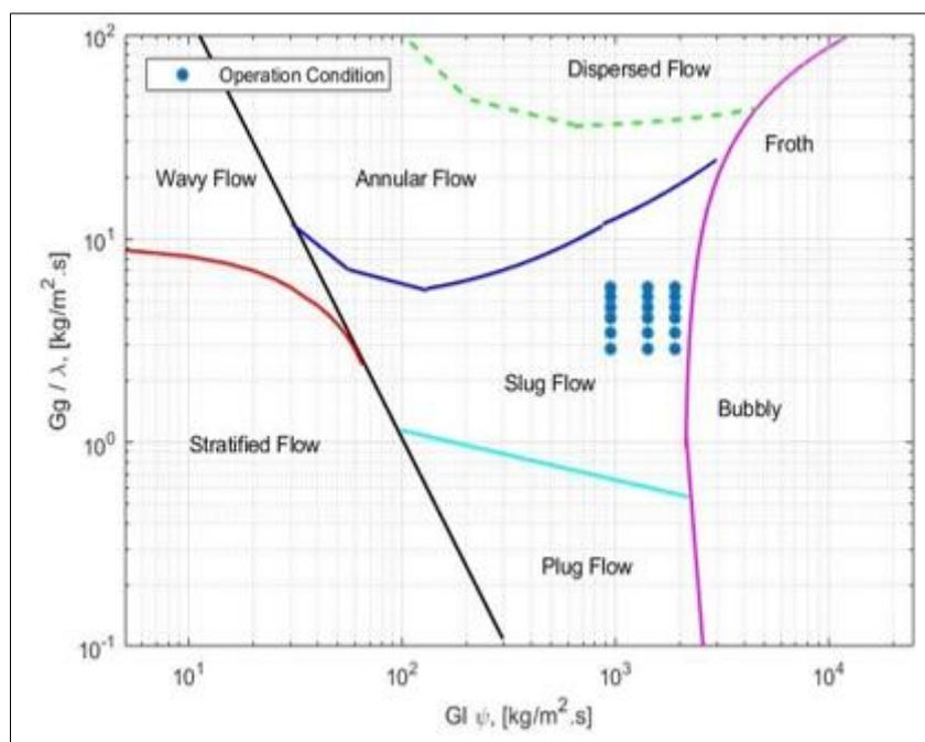
**Figure 4.** Flow pattern map produced by the program based on experimental operating conditions
