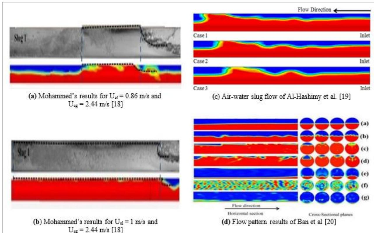
**Figure 3.** Previous research on two-phase air-water flow in a horizontal pipe
