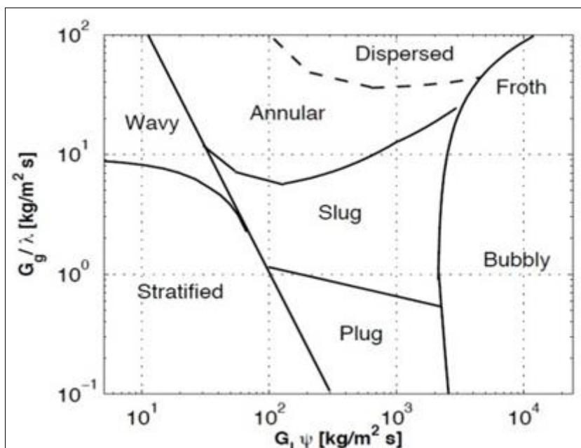
Figure 1. Modified Baker's map in a two-phase horizontal flow pipe [30]
