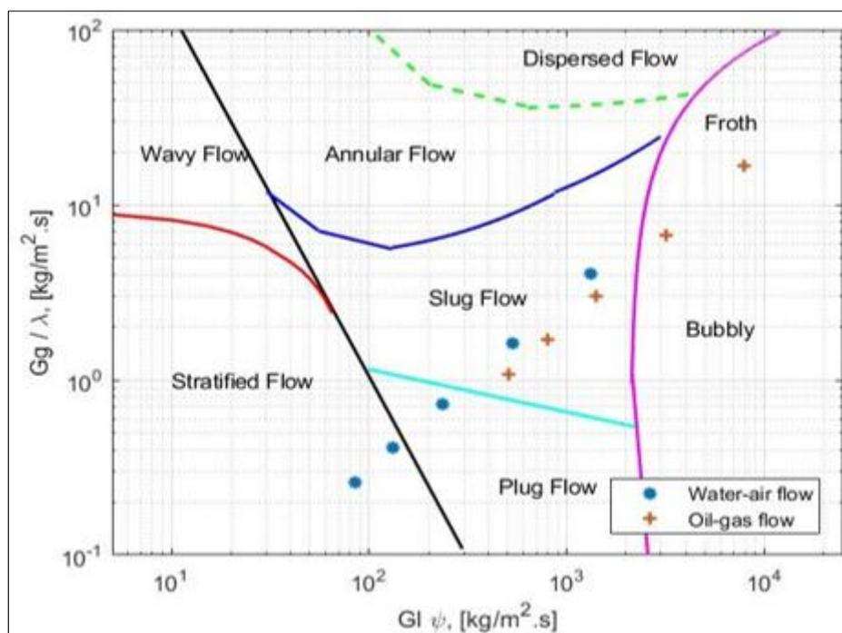
**Figure 6.** Impact of pipe diameters and fluid properties on flow pattern map
