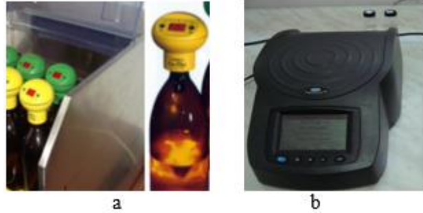
Fig. 2. Laboratory used equipment's [13]: a OxiTop, b Odyssey DR/2500
