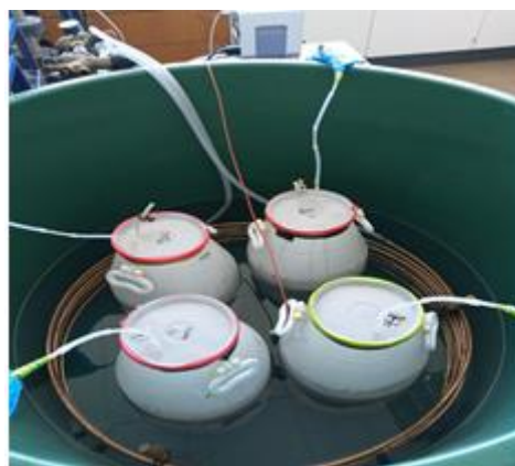
Fig. 2 Laboratory pilot for anaerobically fermentation of biological sludge
