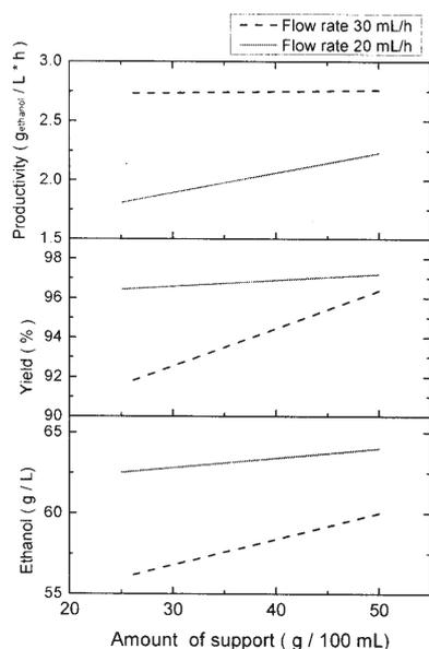
Fig. 6. The influence of the quantity of support on the ethanol concentration, productivity, and the yield of sugars transformation into ethanol temperature 32.5 °C, for two flow rates of the molasses solution
