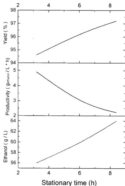
Fig. 4. The influence of the stationary time on the ethanol concentration, productivity and on the real yield of sugars transformation into ethanol, initial molasses concentration 242 g/L, temperature 32.5 °C.
