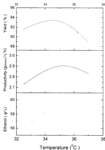
Fig. 7. The influence of fermentation temperature on the ethanol concentration, productivity, and the real yield of sugars transformation into ethanol, stationary time 4 h, molasses concentration 242 g/L, support quantity 25 g/100 mL fermentation medium
