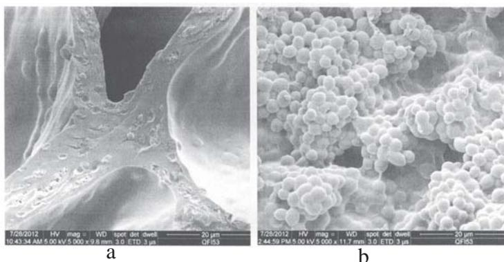
Fig. 3. Sample 5 after 48 h of incubation into the molasses solution, section view (a) and outer surface (b)
