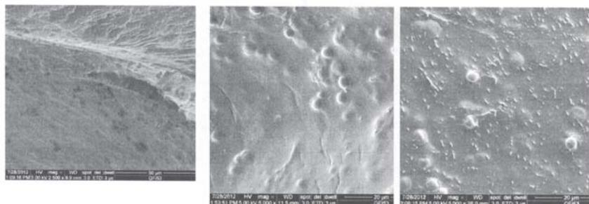
Fig. 2. Electron microscopic scanning images of the samples kept only in water (detailed images of the walls surface)
