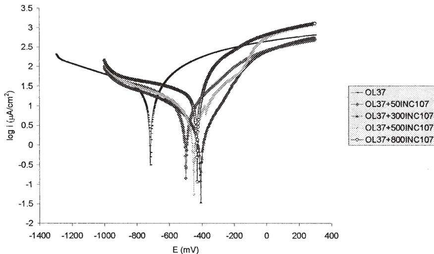
Fig. 1. Polarization curves for OL37 steel in condensed water with and without inhibitor INCOR107
