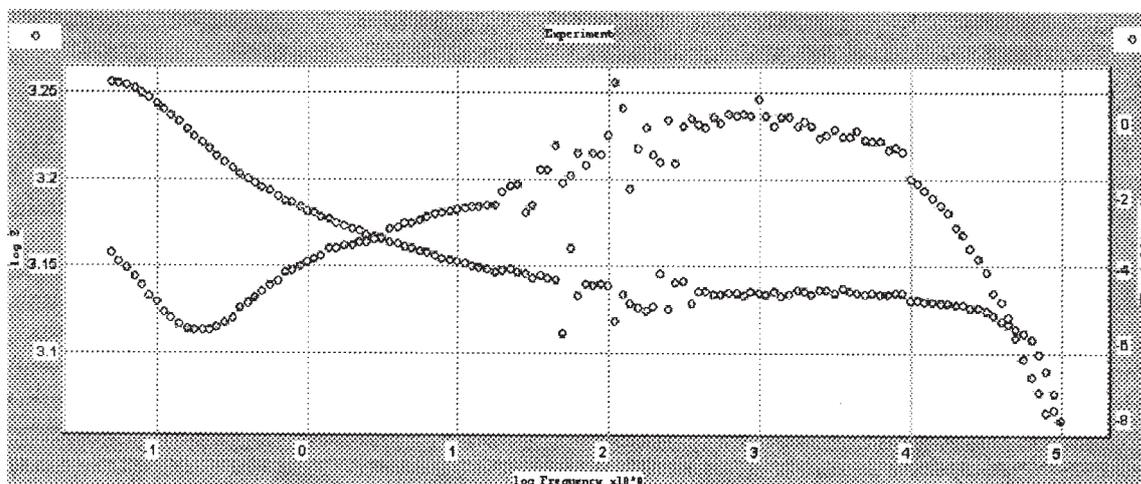
Fig. 3. Bode diagram for OL37 steel in condensed water
