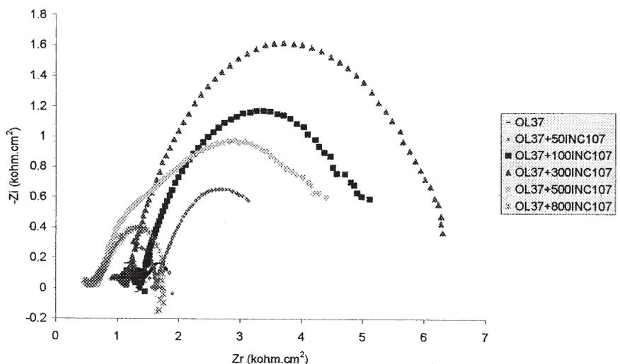
Fig. 2. Nyquist diagram for OL37 steel in condensed water with and without inhibitor INCOR107, at potential in open circuit
