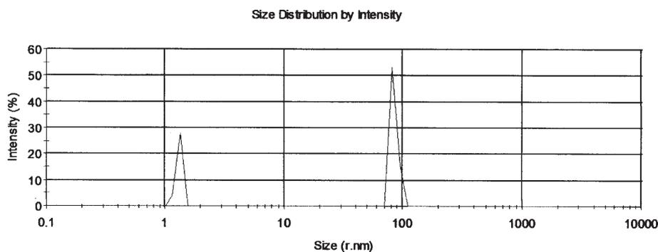
Fig. 2. Particles size distribution of the synthesized silica based support S2 (DLS)
