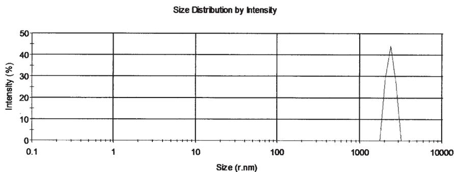
Fig. 1. Particles size distribution of the synthesized silica based support S1 (DLS)
