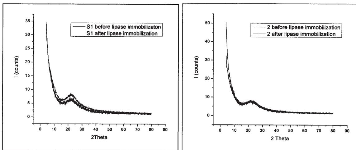
Fig. 7. XRD pattern of sample (S1, S2) before and after lipase immobilization
