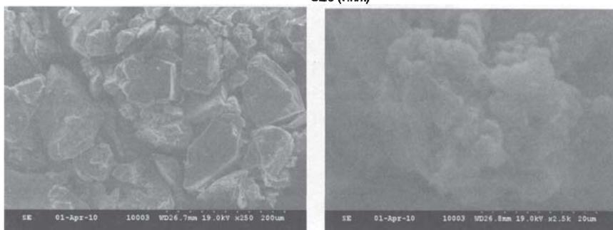
Fig. 3. SEM images of sample S1 before and after lipase immobilization
