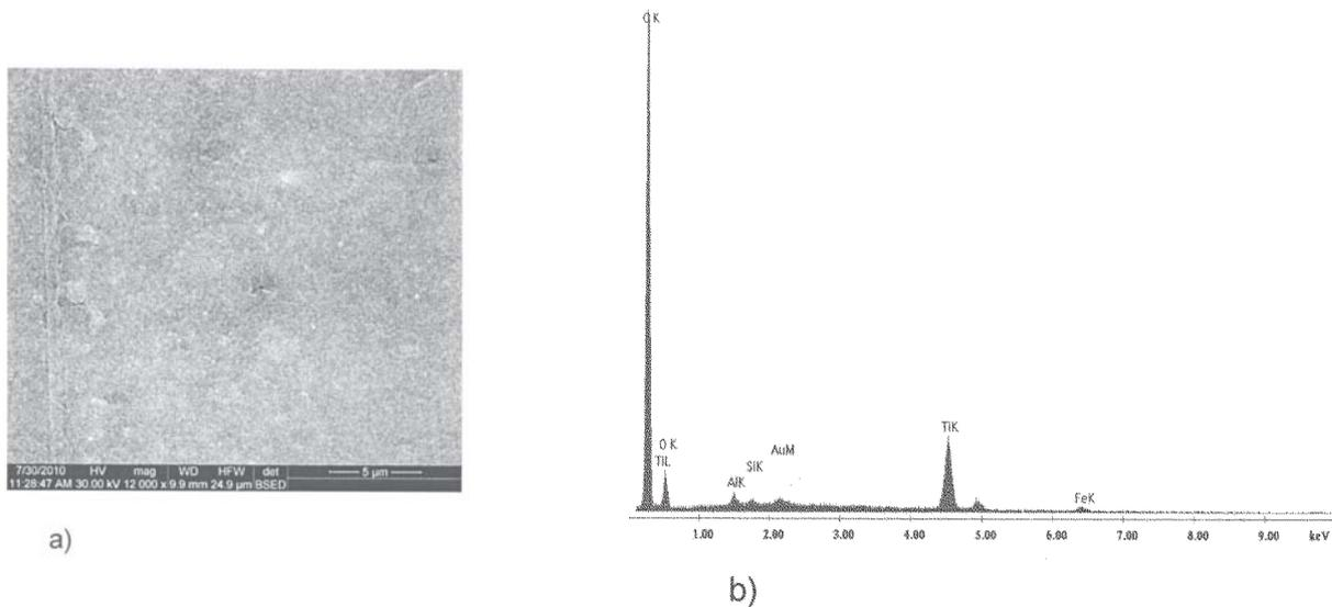
Fig.6. Dried transparent polymeric film containing sample P2; a) SEM image (X 12000) using EDT and b) elemental composition using EDAX
