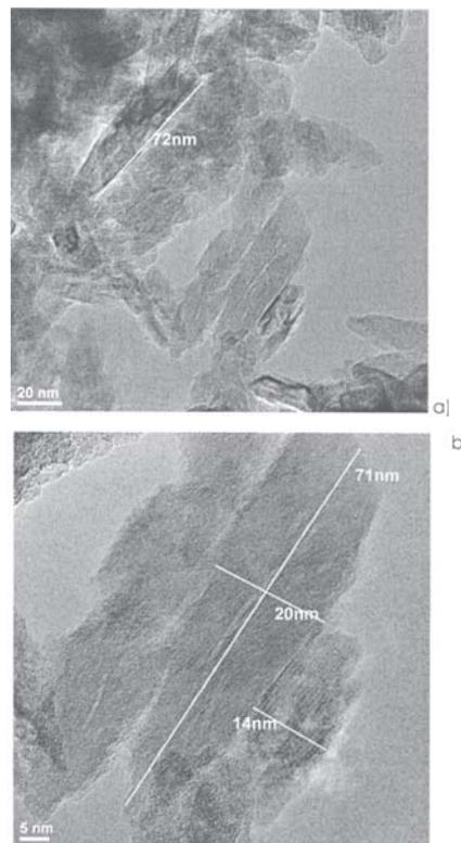
Fig. 2. Size and shape of crystals of sample P1, performed by TEMBF (image a) and by HRTEM (image b)
