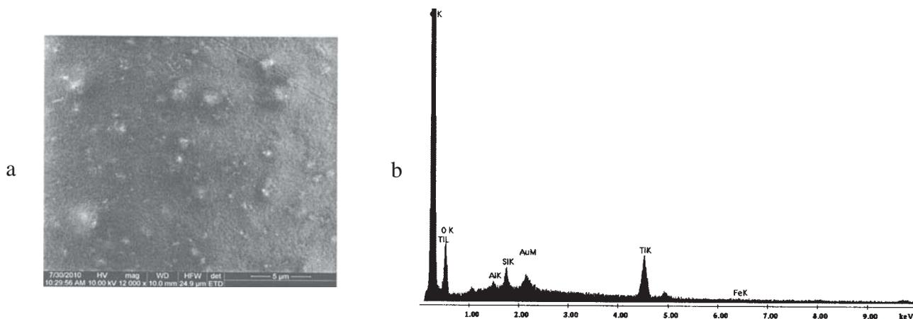
Fig 4. Dried polymeric film containing sample P1; a) EDAX results and b) SEM image (X 12000) using secondary electron detector (ETD)
