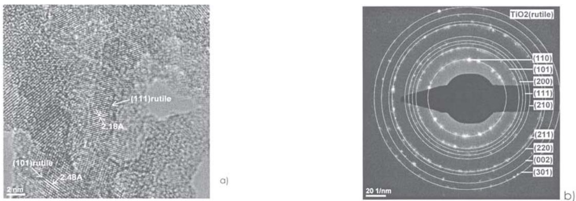
Fig.3 Sample P1; a) HRTEM image with crystallographic planes (101), (111); b) SAED pattern associated to site from image a)
