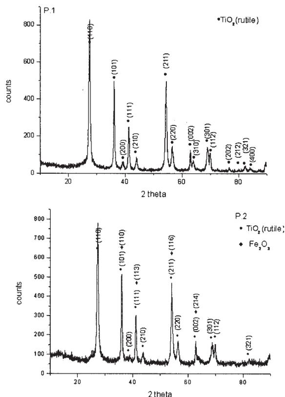
Fig.1 XRD pattern for Sample P1 (iron doped TiO<sub>2</sub>) and Sample P2 (mixture rutile and Fe<sub>2</sub>O<sub>3</sub>)
