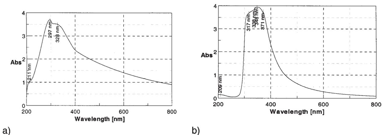
Fig.7. UV Vis spectra for dried film containing 2% w/w iron doped  $\text{TiO}_2$  presented in graph a) and mixture of nano rutile and nano iron oxide ( $\text{Fe}_2\text{O}_3$ ) showed in b)
