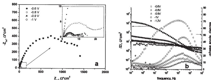
Fig. 8. Nyquist (a) and Bode (b) diagrams on Pt electrode from  $\text{ChCl}$ -ethylene glycol + 8 mM  $\text{CoCl}_2$ , 60°C, at various polarization potentials
