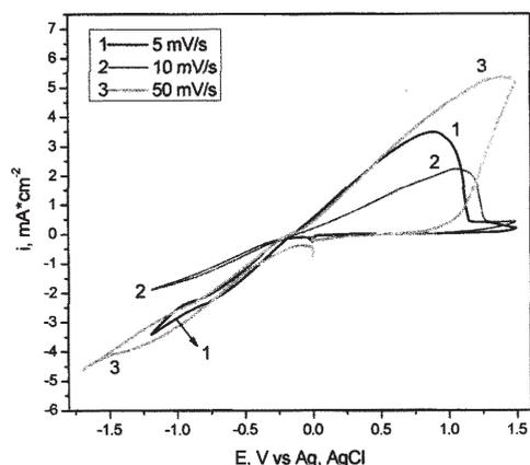
Fig. 3. Cyclic voltammograms on Pt at 25°C for 50 mM  $\text{K}_2[\text{Sb}_2(\text{tartrate})_2]$  dissolved in ethylene glycol at different scan rates
