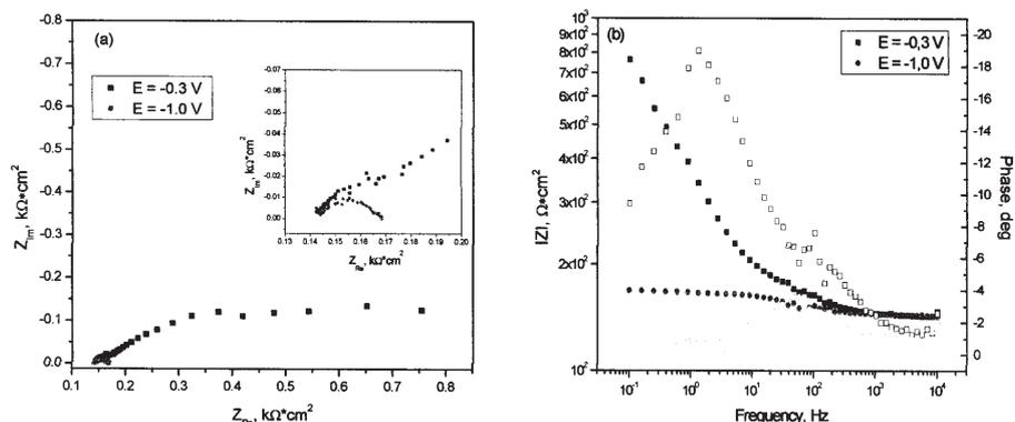
Fig. 2. Nyquist (a) and Bode (b) diagrams on Pt electrode from ethylene glycol + 264 mM  $\text{CoCl}_2$ , 25°C, at various polarization potentials
