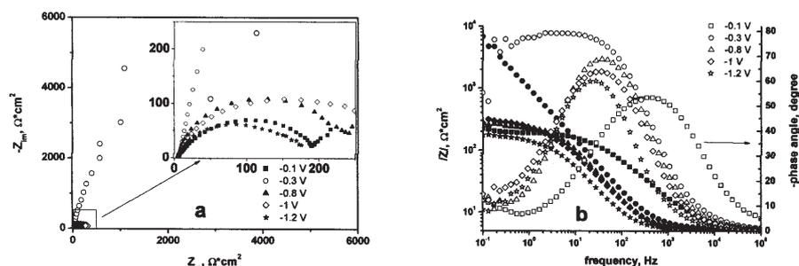
Fig. 14. Nyquist (a) and Bode (b) diagrams on Pt electrode from ChCl-ethylene glycol + 8 mM  $\text{CoCl}_2$  + 4 mM  $\text{SbCl}_3$ , 60°C, at various polarization potentials
