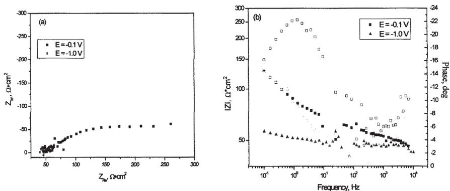
Fig. 4. Nyquist (a) and Bode (b) diagrams on Pt electrode from ethylene glycol + 50 mM  $\text{K}_2[\text{Sb}_2(\text{tartrate})_2]$ , 25°C, at various polarization potentials
