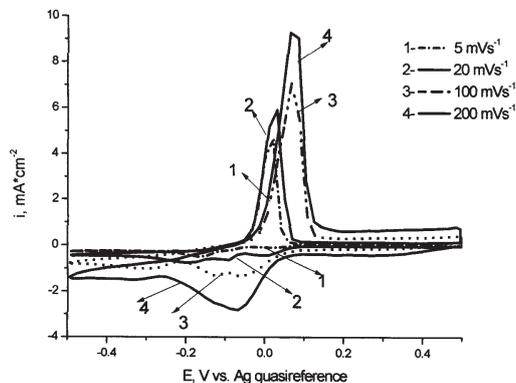
Fig. 9. Cyclic voltammograms on Pt at 60°C for 9 mM  $\text{SbCl}_3$  dissolved in ChCl-ethylene glycol (1:2 moles) eutectic at different scan rates
