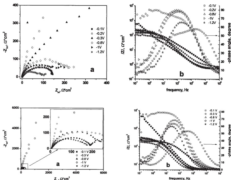
Fig. 13. Nyquist (a) and Bode (b) diagrams on Pt electrode from ChCl-ethylene glycol + 4 mM  $\text{CoCl}_2$  + 9 mM  $\text{SbCl}_3$ , 60°C, at various polarization potentials
