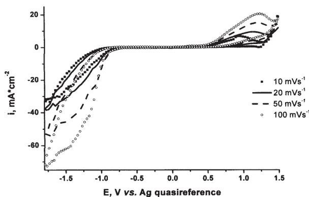
Fig. 7. Cyclic voltammograms on Pt at 60°C for 8 mM  $\text{CoCl}_2$  dissolved in  $\text{ChCl}$ -ethylene glycol (1:2 moles) eutectic at different scan rates
