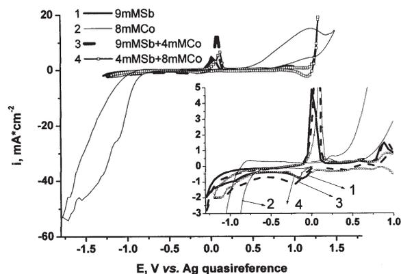
Fig. 12. Comparative CV curves on Pt at 60°C for single  $\text{CoCl}_2$  or  $\text{SbCl}_3$  and for both  $\text{CoCl}_2$  and  $\text{SbCl}_3$  dissolved in ChCl-ethylene glycol (1:2 moles) eutectic; scan rate  $50 \text{ mVs}^{-1}$
