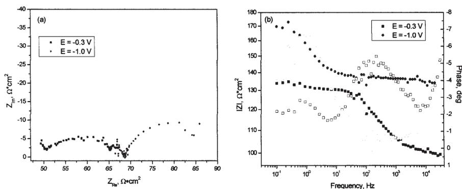
Fig. 6. Nyquist (a) and Bode (b) diagrams on Pt electrode from ethylene glycol + 50 mM  $\text{K}_2[\text{Sb}_2(\text{tartrate})_2]$ , 25°C, at various polarization potentials
