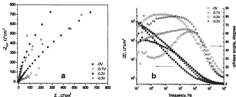
Fig. 10. Nyquist (a) and Bode (b) diagrams on Pt electrode from ChCl-ethylene glycol +  $9\text{ mM}\ \text{SbCl}_3$ ,  $60^\circ\text{C}$ , at various polarization potentials
