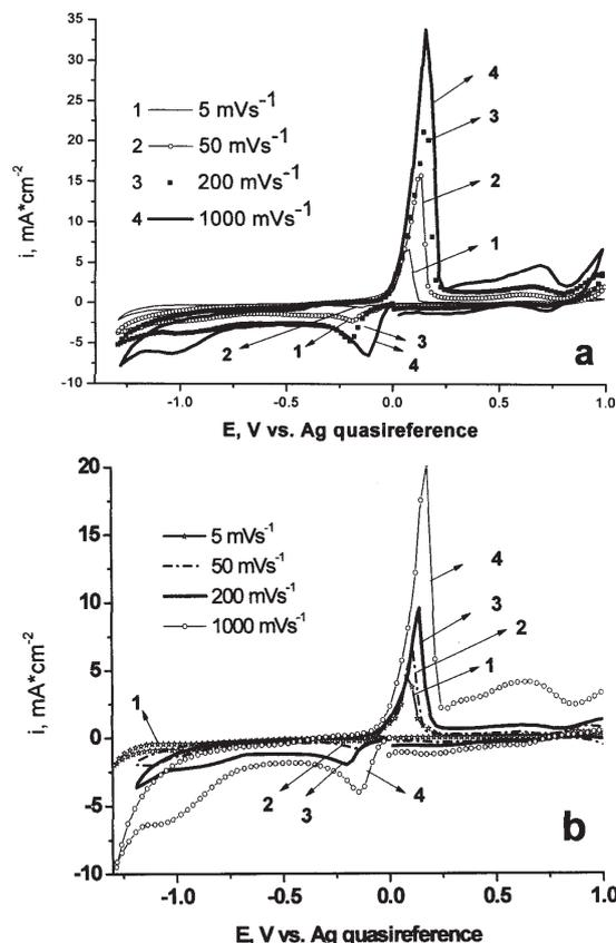
Fig. 11. Comparative CV curves on Pt at  $60^\circ\text{C}$  for both  $\text{CoCl}_2$  and  $\text{SbCl}_3$  dissolved in ChCl-ethylene glycol (1:2 moles) eutectic: (a)  $4\text{ mM}\ \text{CoCl}_2$  and  $9\text{ mM}\ \text{SbCl}_3$ ; (b)  $8\text{ mM}\ \text{CoCl}_2$  and  $4\text{ mM}\ \text{SbCl}_3$
