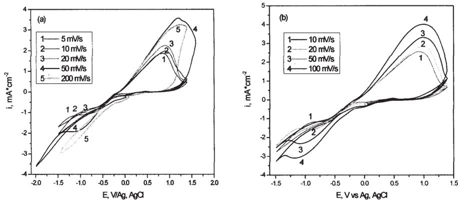
Fig. 5. Comparative CV curves on Pt at 25°C for both  $\text{CoCl}_2$  and  $\text{K}_2[\text{Sb}_2(\text{tartrate})_3]$  dissolved in ethylene glycol: (a) 132 mM  $\text{CoCl}_2$  and 25 mM  $\text{K}_2[\text{Sb}_2(\text{tartrate})_2]$  (b) 270 mM  $\text{CoCl}_2$  and 25 mM  $\text{K}_2[\text{Sb}_2(\text{tartrate})_2]$
