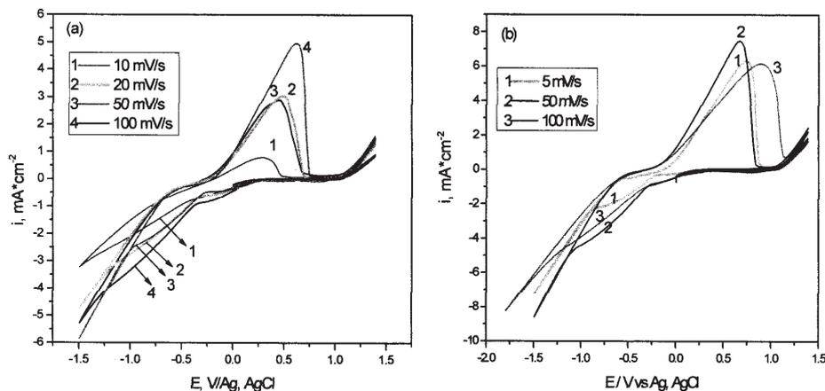
Fig. 1. Cyclic voltammograms on Pt at 25°C for 264 mM  $\text{CoCl}_2$  (a) and 540 mM  $\text{CoCl}_2$  (b), dissolved in ethylene glycol at different scan rates
