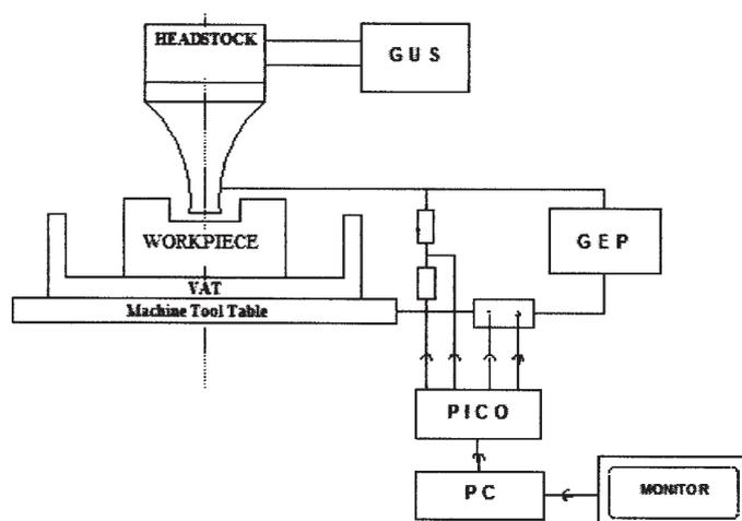
Fig. 1 Technological equipment for the EDMUS non-conventional technology: (GUS-ultrasonic generator, GEP-isoenergetic impulse generator, PICO-oscilloscope)
