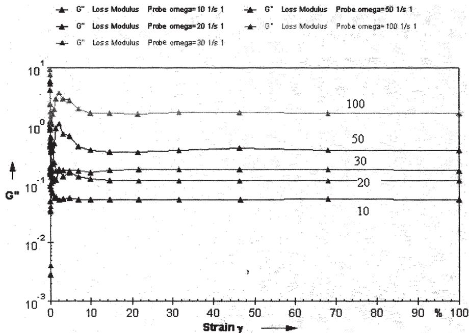
Fig. 6 Amplitude tests at different frequency values (written on curves, in  $s^{-1}$ ), for the used liquid, at a temperature of  $20^{\circ}C$
