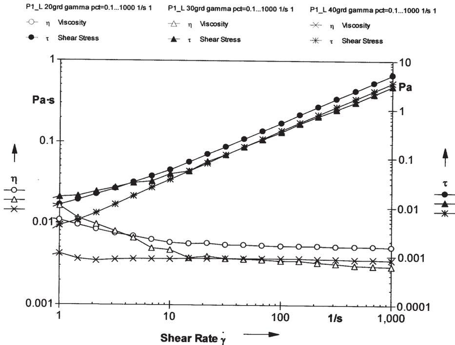
Fig. 4 Influence of the temperature on the flow curves  $\tau=f(\dot{\gamma})$  (bold symbols) and  $\eta=f(\dot{\gamma})$  of the used dielectric liquid
