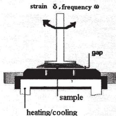
Fig. 2. Scheme of the plane-plane device used for rheological studies
