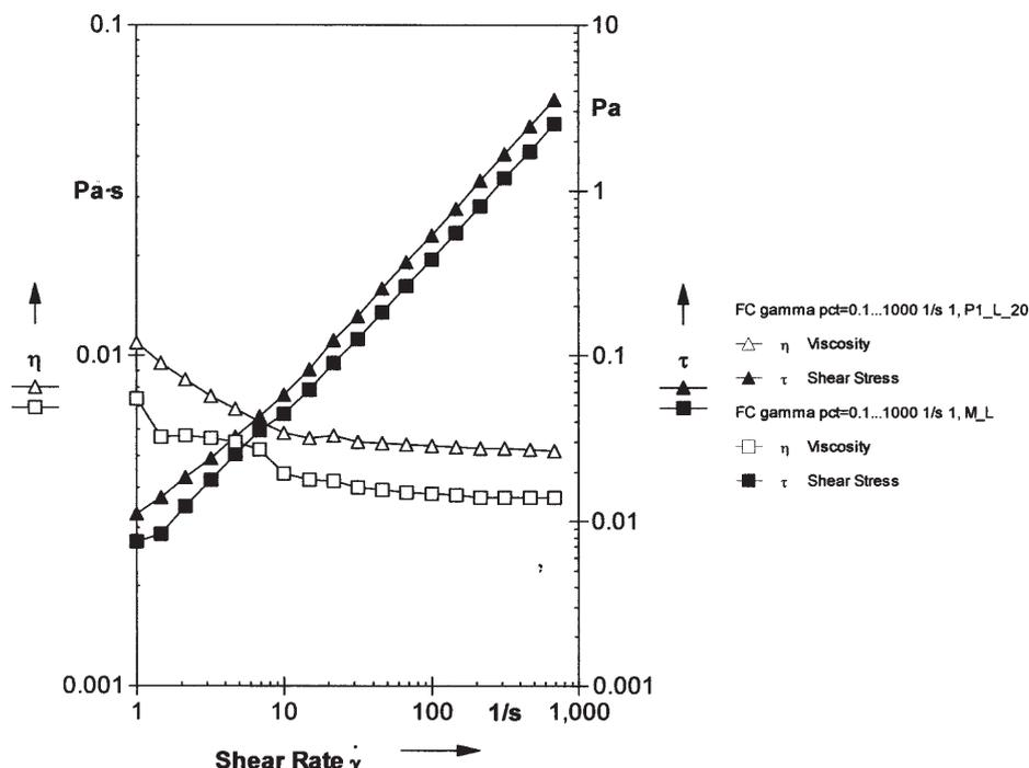
Fig. 3 Rheological functions  $\tau=f(\dot{\gamma})$  (bold symbols) and  $\eta=f(\dot{\gamma})$  for the fresh liquid ( $\square$ ) and the used liquid ( $\Delta$ ), respectively, at 20°C
