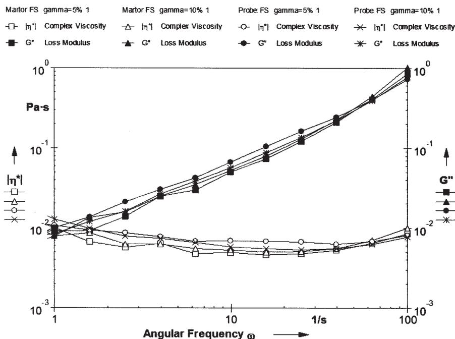
Fig. 5 The variation of the viscous modulus  $G''$  and complex viscosity  $\eta^*$  as a function of the oscillation frequency for the fresh dielectric liquid (Martor) and for the used dielectric liquid (Probe), by using two different values for the oscillation amplitude ( $\gamma$ ): 5% and 10%
