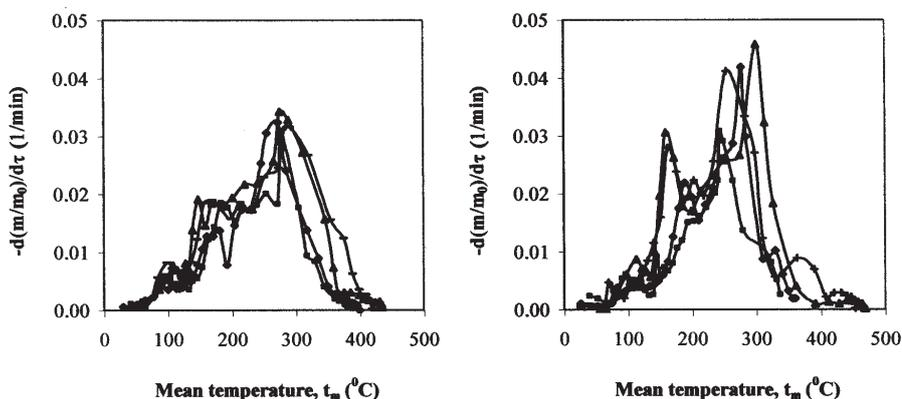
Fig. 5. Mass loss rate versus logarithmic mean temperature ( $\blacklozenge$  exp 1,  $\blacksquare$  exp 2,  $\blacktriangle$  exp 3,  $-$  exp 4,  $\diamond$  exp 5,  $\square$  exp 6,  $\Delta$  exp 7,  $+$  exp 8)
