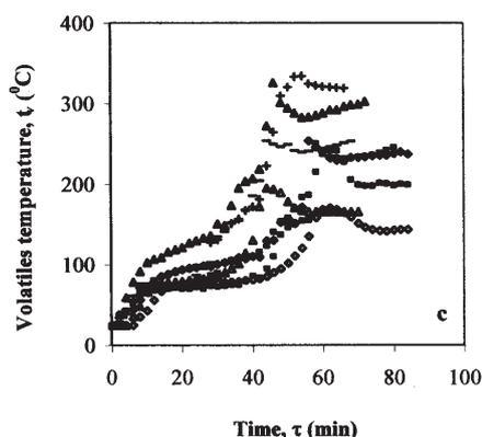
Fig. 4. Time variation of temperature of: a) material bed centre; b) column wall; c) volatiles ( $\blacklozenge$  exp 1,  $\blacksquare$  exp 2,  $\blacktriangle$  exp 3,  $-$  exp 4,  $\diamond$  exp 5,  $\square$  exp 6,  $\Delta$  exp 7,  $+$  exp 8)
