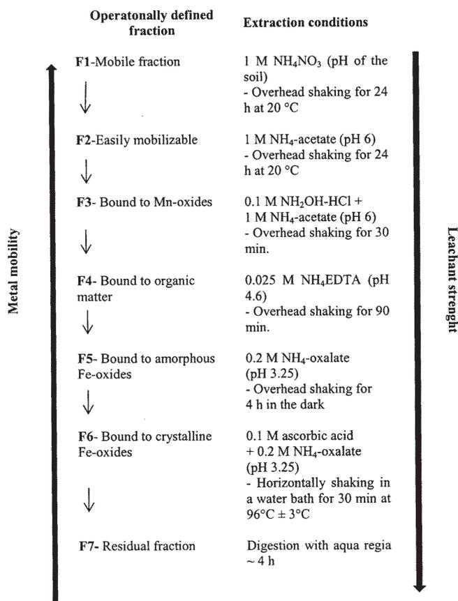
Fig. 1. Relationship between metal mobility in the different operationally-defined phases and leachant strenght of chemical reagents used for Zeien- Brummer SEP [24]
