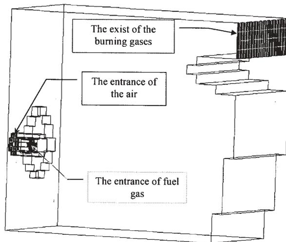
Fig.1. The geometrical model of the furnace
