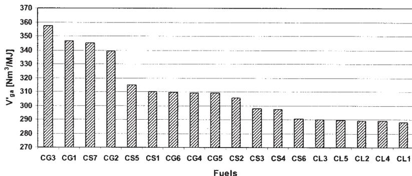
Fig. 2. Values of the normalized volumes of combustion gases
