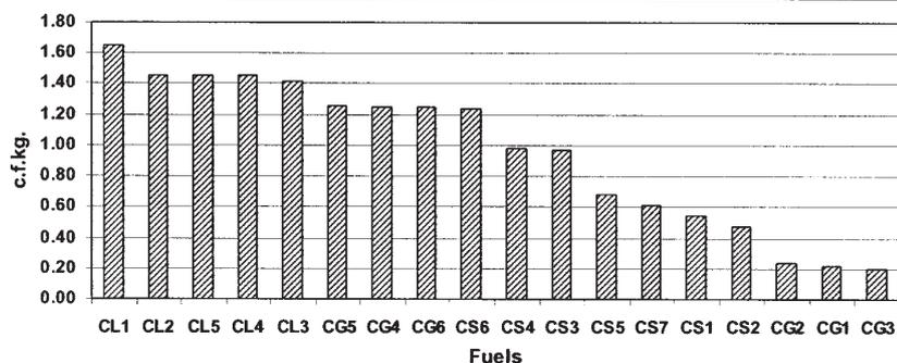
Fig. 1. Values of the inferior heat power equivalent expressed in conventional fuel kilogram (c.f.kg.)
