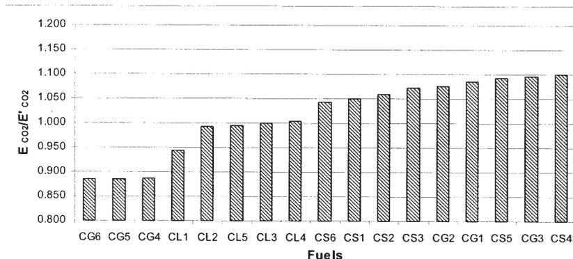
Fig. 3. The emissive power of CO<sub>2</sub> referred to black oil.
