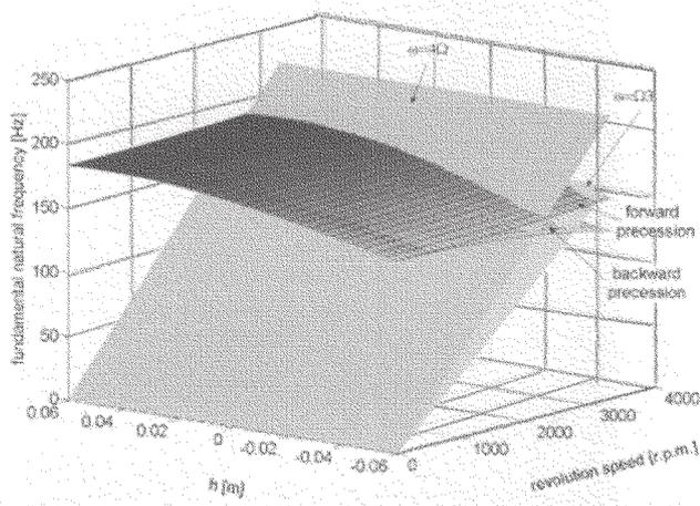
Fig. 5. Variation of fundamental natural frequency depending on the rotation speed and on the position of the fixing point of the basket on the shaft with respect to the centre of mass
