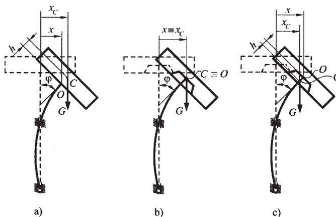
Fig. 1. The position of the fixing point of the basket with respect to the centre of mass in the case of a centrifuge with vertical axis
