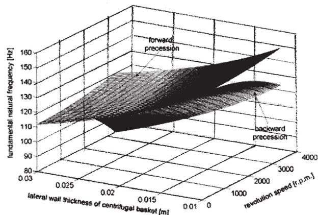
Fig. 6. Variation of fundamental natural frequency depending on the rotation speed and on the thickness of the side wall of the basket
