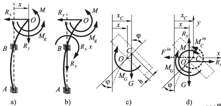
Fig. 2. The calculus of reactions in the fixing point of the basket on the shaft. The action of the gyroscopic moment
