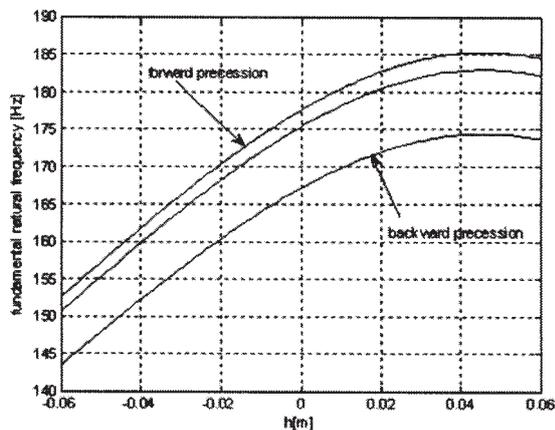
Fig. 4. Variation of fundamental natural frequency depending on the position of the fixing point of the basket on the shaft in comparison with the centre of mass
