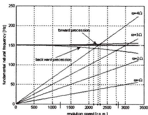
Fig. 3. Variation of fundamental natural frequency depending on the rotation speed for a basket wall thickness of 0.01 m
