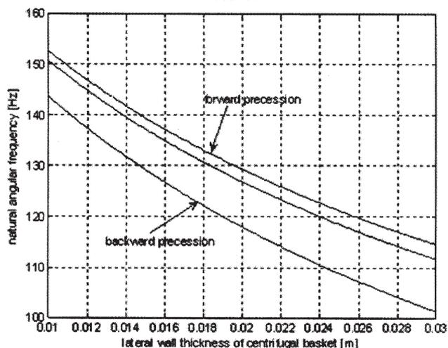
Fig. 7. Variation of fundamental natural frequency depending on the thickness of the side wall of the basket
