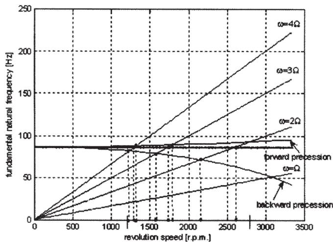
Fig. 8. Variation of fundamental natural frequency depending on the speed, for a basket wall thickness of 0.03 m.
